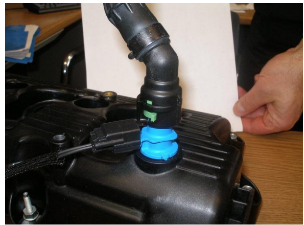
Assembled PCV system
