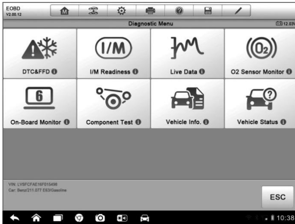
Figure 4-14 Sample OBD II Diagnostic Menu
