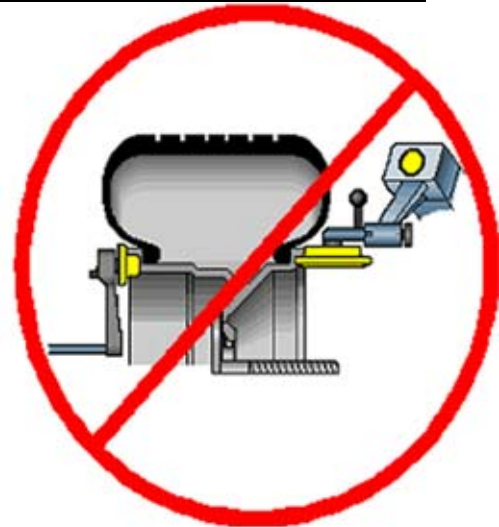
INCORRECT POSITION FOR MEASURING RIM RUNOUT
