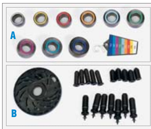
The low-taper of a direct-fit, dual-taper collet (versus the high-taper cone) offers better hub bore contact and prevents bottoming out on recently popular outer hubcap alloy wheel bore designs.
