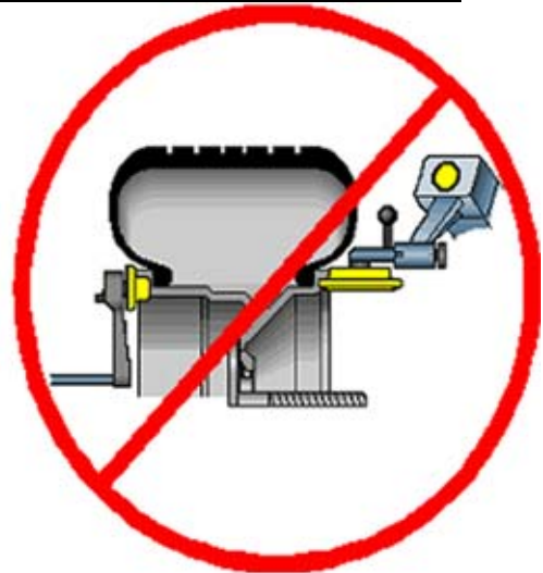
INCORRECT POSITION FOR MEASURING RIM RUNOUT
