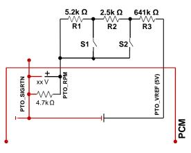
SAMPLE PROCEDURE: THREE-SPEED SEIC (1300, 1800 AND 2400 RPM) WITH 3-POSITION SWITCH SCENARIO 1 (2400 RPM): Choose a resistor for the highest of the three desired speeds, 2400 RPM in this example, which requires a 641-Ohm resistor (per the resistor tables). This will be referred to as R3. When the switch is in Position 3, the total resistance between PTO\_VREF and PTO\_RPM is R3 = 641 Ohms. R3 = 641 Ohms.
