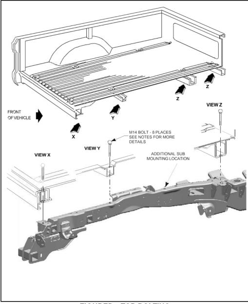
MOUNTING TECHNIQUES FOR PICK-UP BOX REMOVAL
