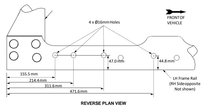
Four holes are in each frame-rail (in the bottom flange). These holes are to facilitate the installation of aftermarket trailer hitches. Aftermarket hitch load ratings are the responsibility of the aftermarket hitch manufacturer. The maximum trailer tow rating which is published in the Ford RV & Trailer Tow Guide must not be exceeded.
