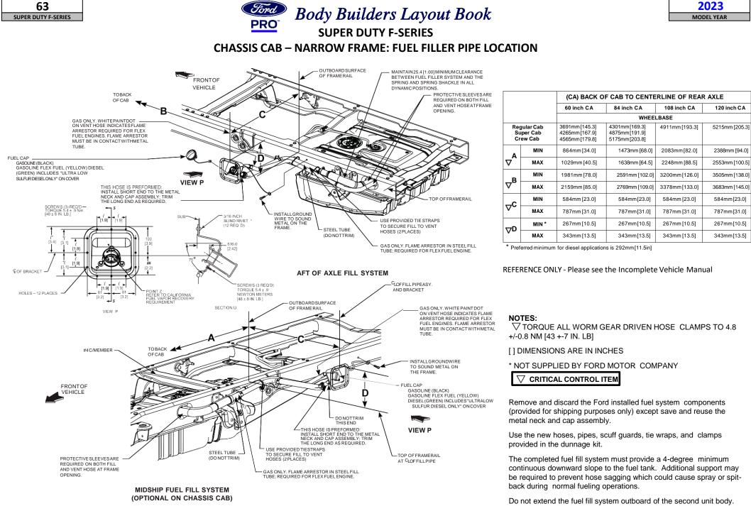
The installation of Tube Extension F81A-9B149-HA will permit the location aft-of-axle fuel fill housing to be no further rearward than the centerline of the fill hose as it passes through the frame.
