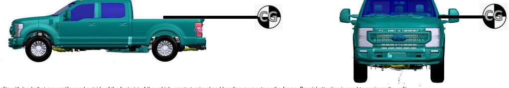
Upfits with loads that are cantilevered outside of the footprint of the vehicle create torsional and bending moments on the frame. Special attention is need to engineer the upfit
