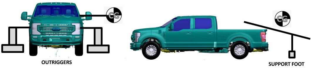
Upfits that include user deployed support structures to react loads at the ground such as outriggers and support feet will create torsional and bending moments on the frame if the user deploys the support structures incorrectly. Special attention is needed to ensure proper use instructions are communicated to the user
