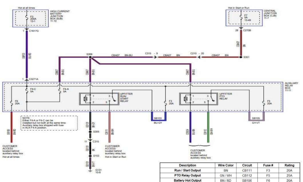
Either F4A or F4C can be installed but not both at the same time. Upfitter Relay Box is shipped with fuse in F4A position.
