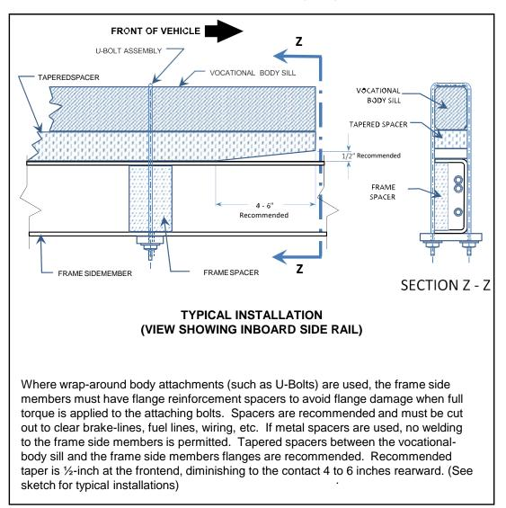
FIGURE C - CHASSIS CAB SUB-MOUNTING SPACER
