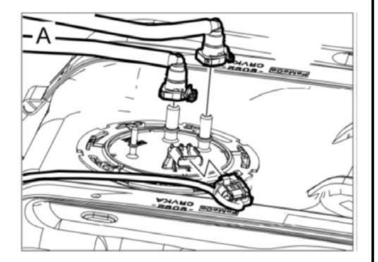
All Super-Duty Chassis Cab fuel tanks (except the aft tank on dual-tank diesels) come equipped with an Auxiliary Fuel Port located in the fuel sender unit on the top of the fuel tank.
