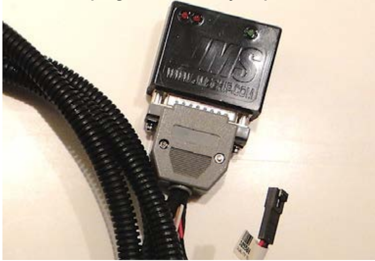
ID the Map Sensor Connectors: Cable is labeled: MAP Only three wires
